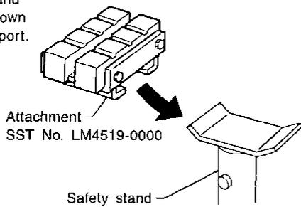
Fit the lower side sill into groove.
