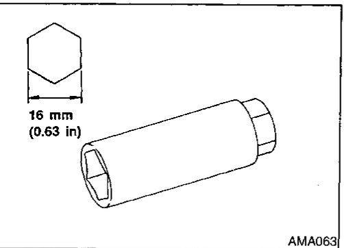
2. Remove spark plugs with spark plug socket.
