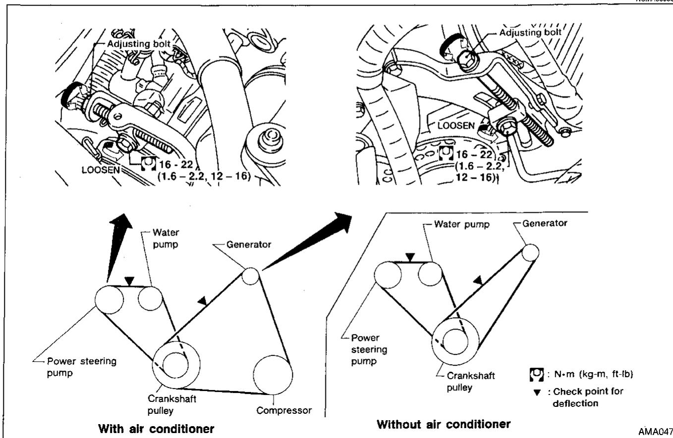
1. Inspect belt for cracks, fraying, wear and oil. If necessary, replace.
