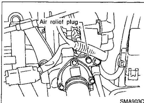
4. Remove cylinder block drain plug and air relief plug.
