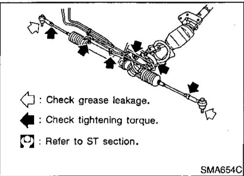
**Checking Steering Gear and Linkage**
