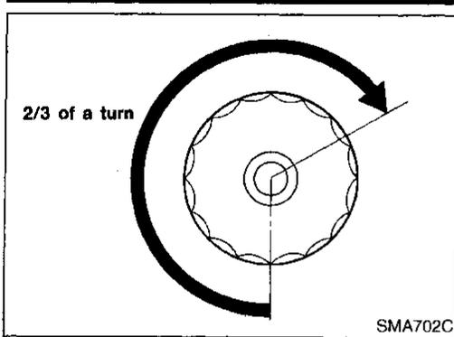
3. Screw in the oil filter until a slight resistance is felt, then tighten an additional 2/3 turn.
