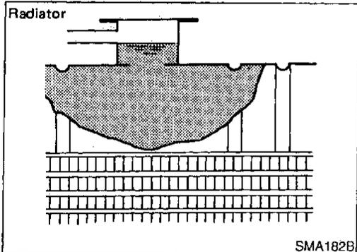
2. Fill radiator slowly with coolant until coolant spills from the air relief plug, then install air relief plug.
