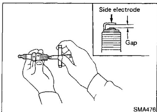
3. Check plug gap of each new spark plug.
