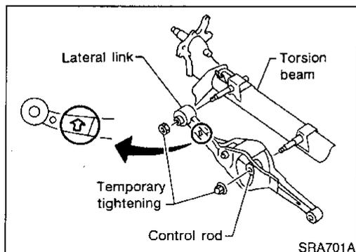
2. Temporarily install lateral link and control rod on torsion beam.
