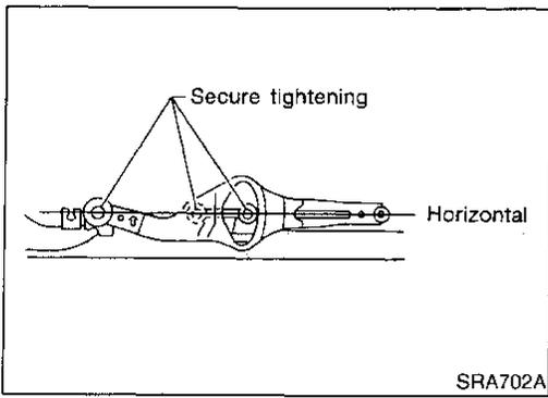
3. Place lateral link and control rod horizontally against torsion beam, and tighten to the specified torque.
