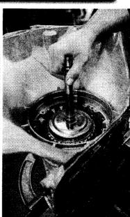
Finally, our 200-4R is starting to look like a full unit. The input shaft is connected to the overdrive assembly. Although the engine's torque reaches fourth gear first, overdrive is not operated until its . band is applied. This causes the direct and forward assemblies to be driven first.
