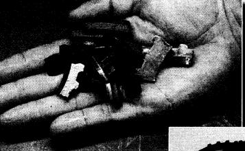
Here are the preferred steels used in the clutch packs. These steels are coated in Kolene, which increases the coefficient of friction, Or, in layman's term's, "bite" on the friction material of the clutches. When a clutch pack engages, high-pressure transmission fluid is sent from the valve body to Squeeze on a set of these Kolene steels. It then locks up with alternating clutch plates that have friction material on them-kind of like a clutch pack sandwich.
