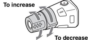
If you need to mount the rotary commander on the right hand side of the steering column, you can reverse the operative direction.
