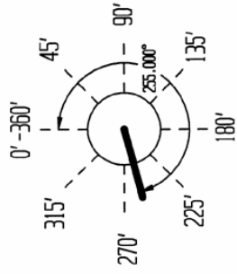
2nd TUBE .1875 HOLES FACE 255 DEGREES
