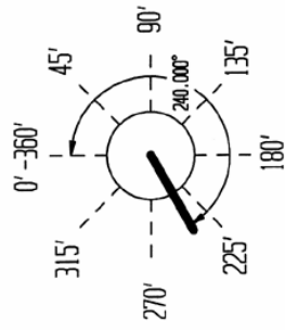
1st TUBE .1875 HOLES FACE 240 DEGREES
